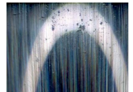
Indentations in raceway caused by particles
