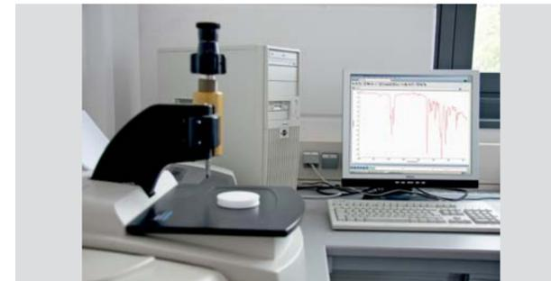
FTIR spectroscopy with ATR technology for non-destructive analysis of the quality composition of organic materials.
